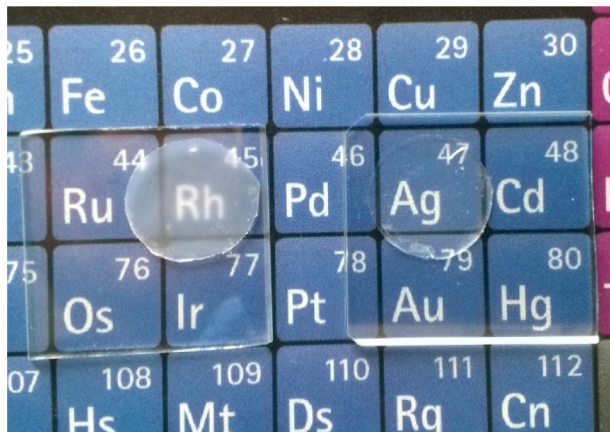
Figure 3. Picture of nonperfect nanocoating (left) and good-performing nanocoating (right).
